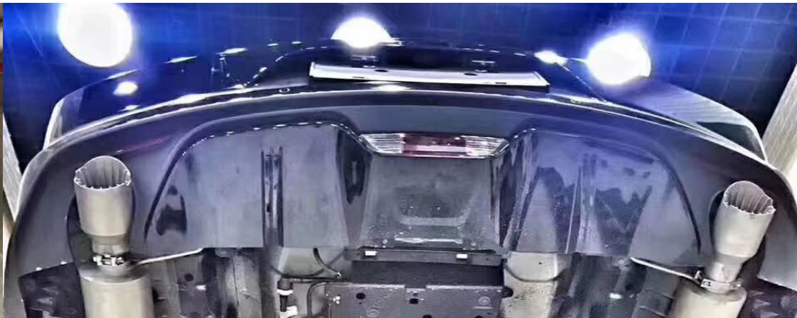
Customized Ford Mustang metal 3D printed exhaust pipes
