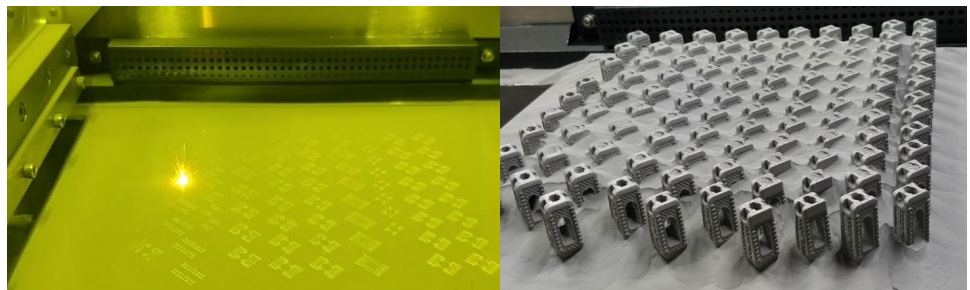
Metal 3D printing process in the chamber
