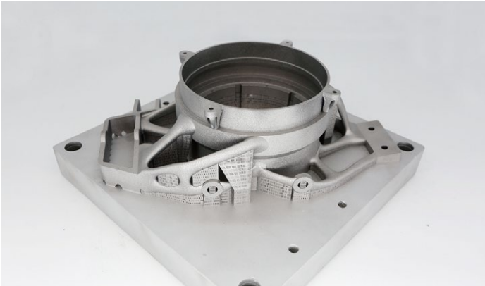
Auto steering column of light weight construction in Aluminum Alloy
